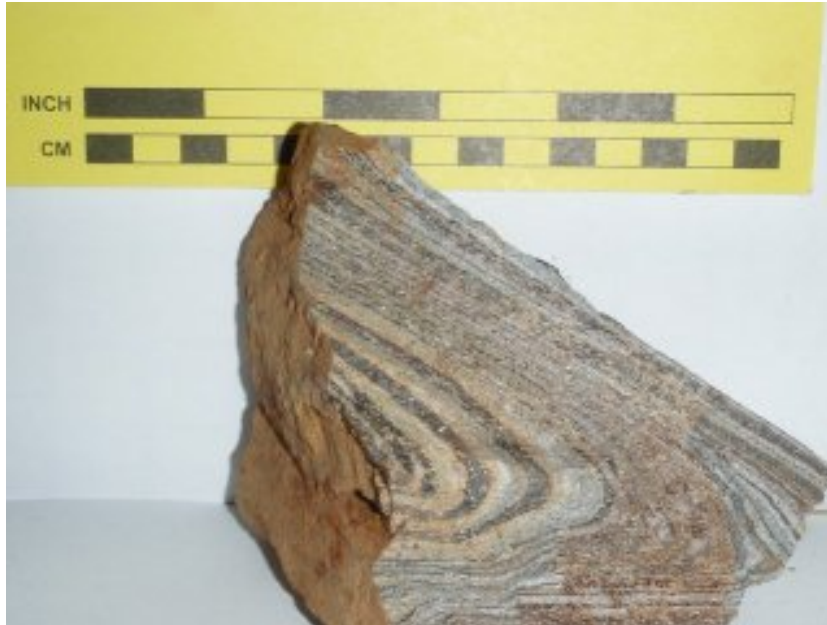
Figure 10. Folded Grade II banded iron formation (BIF) from the Mitzic licence area with thickening of the magnetite bands in the hinges. The steep dip and tight isoclinal folding seen in the field suggests the BIF unit has been significantly thickened may continue at depth.
