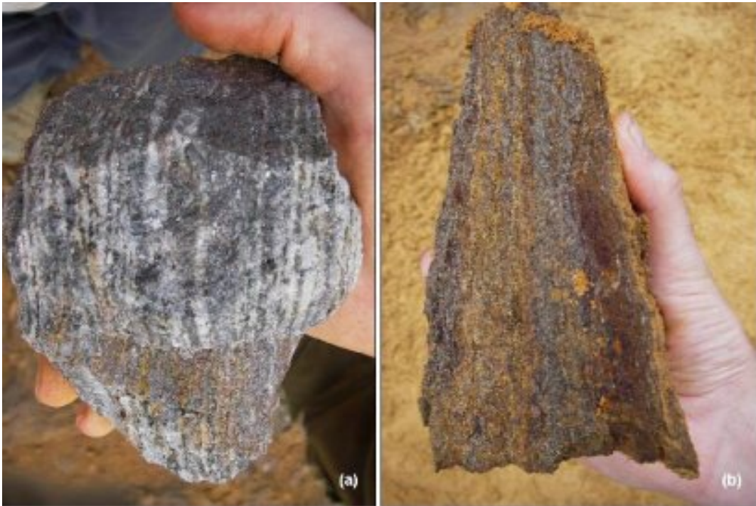
Figure 9. Class I rocks consist of massive, often hematite-stained quartzites with disseminated, moderately to strongly weathered, magnetite grains (magnetite content 1-10 %). Banded Fe-quartzites, with thin (1-2mm) layers of fine-medium grained magnetite (10-15 % magnetite content) which is often moderately oxidised also falls into this class I.
