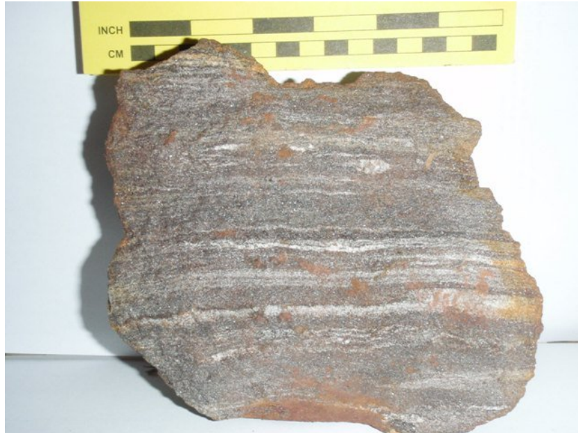
Figure 12. Class III rocks consist of Banded itabirites and BIF's with an estimated magnetite content of 50-75 % magnetite. Segregation banding is the dominant fabric; however the quartz bands are thinner and sometimes slightly discontinuous, compared to the magnetite rich layers.
