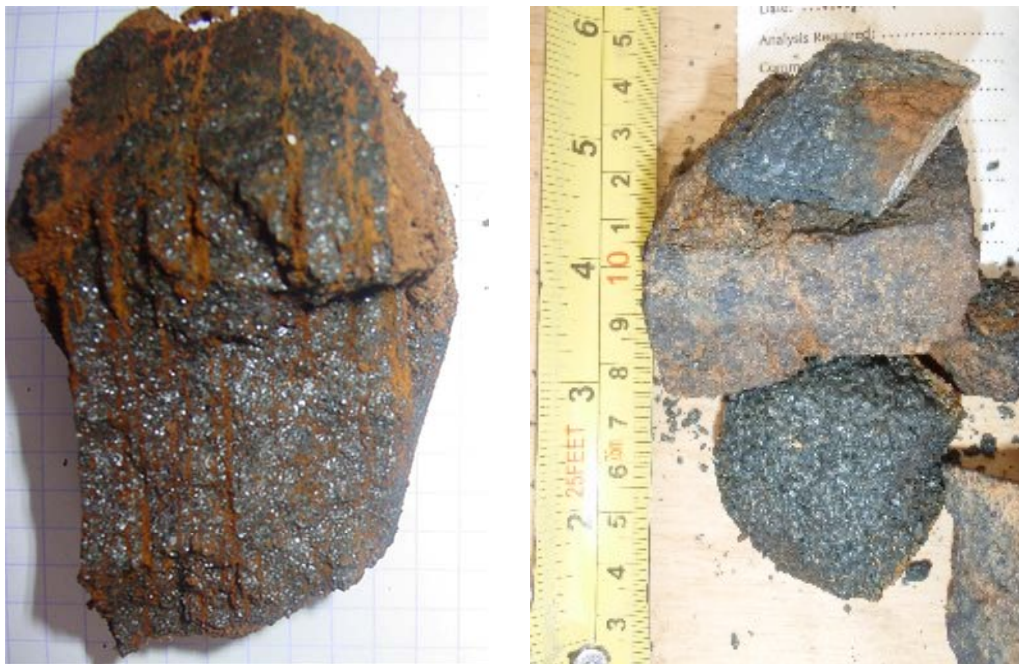
Figure 13. Class IV is defined by complete enrichment of an iron-bearing host. Quartz is absent to rare, with medium to coarse grained, magnetite \pm minor hematite typically forming a massive replacement fabric (>75% magnetite content). In the field this enrichment is seen to occur as pods within a background class II host, or at lithological/structural contacts of iron formation and slivers of ultrabasic assemblages.
