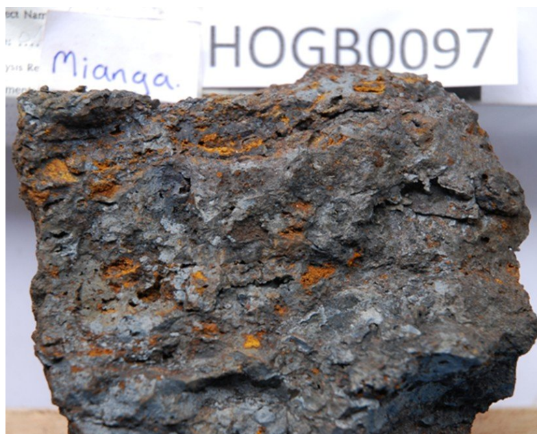
Figure 5. Photo of the sample yielding over 47% manganese. This is thought to possibly represent an enriched zone over a lower grade but more extensive manganese bearing unit within the Proterozoic rocks of the Ogooue Super group.
